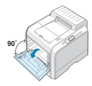
**CAUTION**: If the left cover is not completely open, the top cover release button does not be pressed.
